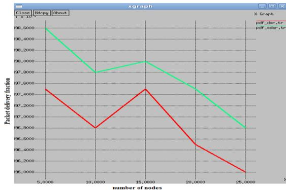
Fig 2. Packet Delivery Fraction vs. Nodes
