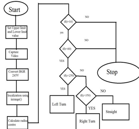
Fig.7, Flow chart of the object tracking system
