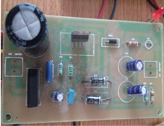
Fig.6, Driver circuit of the system
