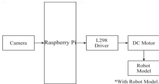
Fig.2, Block Diagram of the object tracking robot
