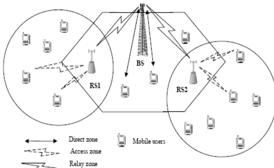
Fig: 2 Structure of WiMAX relay network
