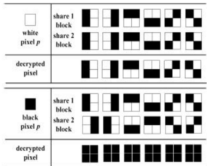
**Fig.1. Construction of (2, 2) VC scheme**
