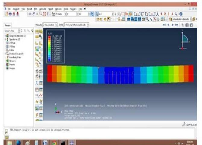
**Fig 5 : Deflected Model Yield Stage from ABAQUS Software**
