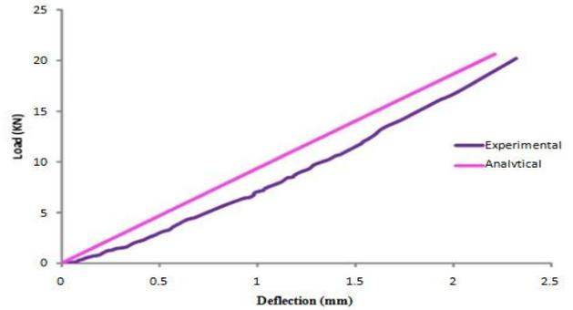
**Fig 14: Comparison of Experimental and ABAQUS Load Vs. Deflection Curve of Toughened Type Glass without Reinforcement**
