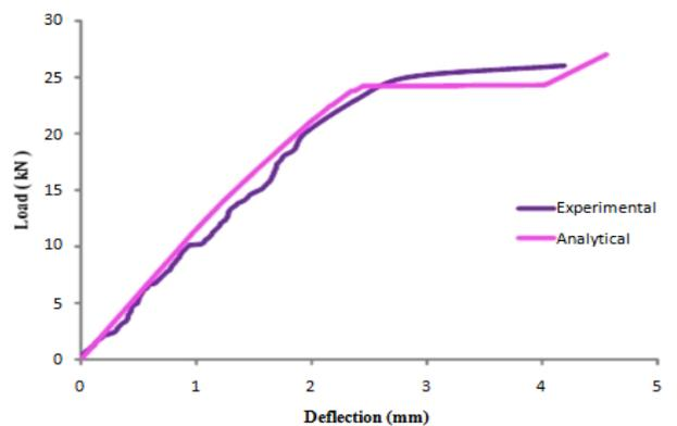
**Fig 16: Comparison of Experimental and ABAQUS Load Vs. Deflection Curve of Toughened Type Glass with 1.2mm Thickness S.S Plate Reinforcement**
