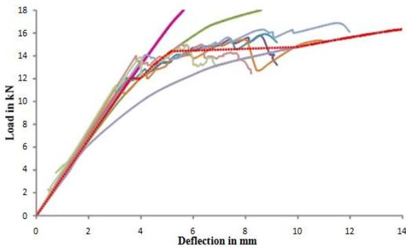
**Fig 7: Interconnected Load vs. Deflection in All Three Stages of Failure in the Middle of the Span**
