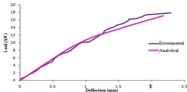
**Fig 13: Comparison of Experimental and ABAQUS Load Vs. Deflection Curve of Annealed Type Glass with 1.2mm Thickness S.S Plate Reinforcement**
