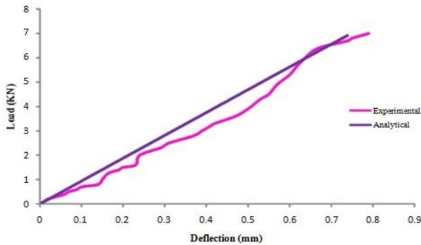
**Fig 11: Comparison of Experimental and ABAQUS Load Vs. Deflection Curve of Annealed Type Glass without Reinforcement**
