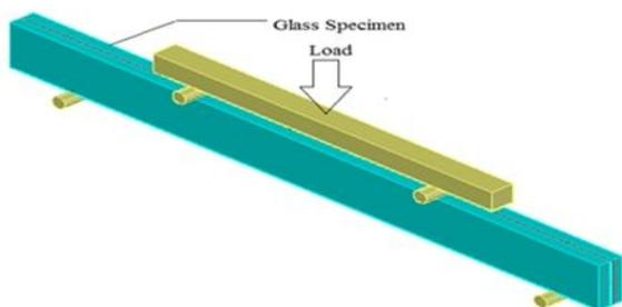
**Fig 8 : Four-Point Bending Test**
