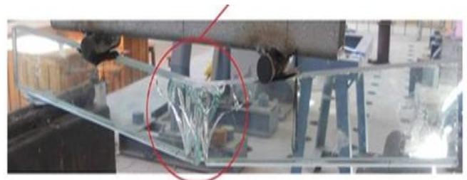
**Fig 9: Failure Pattern of Annealed Glass**
