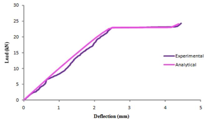
**Fig 15: Comparison of Experimental and ABAQUS Load Vs. Deflection Curve of Toughened Type Glass with 0.36mm Thickness S.S Plate Reinforcement**
