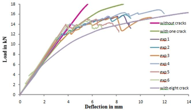
**Fig 6 : Comparison of Load Vs. Deflection in the Middle of the Span**
