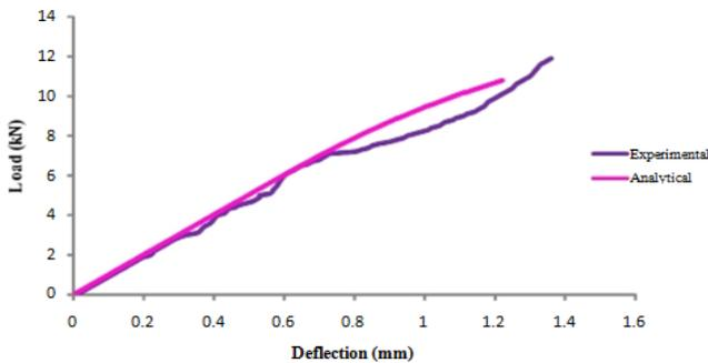
**Fig 12: Comparison of Experimental and ABAQUS Load Vs. Deflection Curve of Annealed Type Glass with 0.36mm Thickness S.S Plate Reinforcement**
