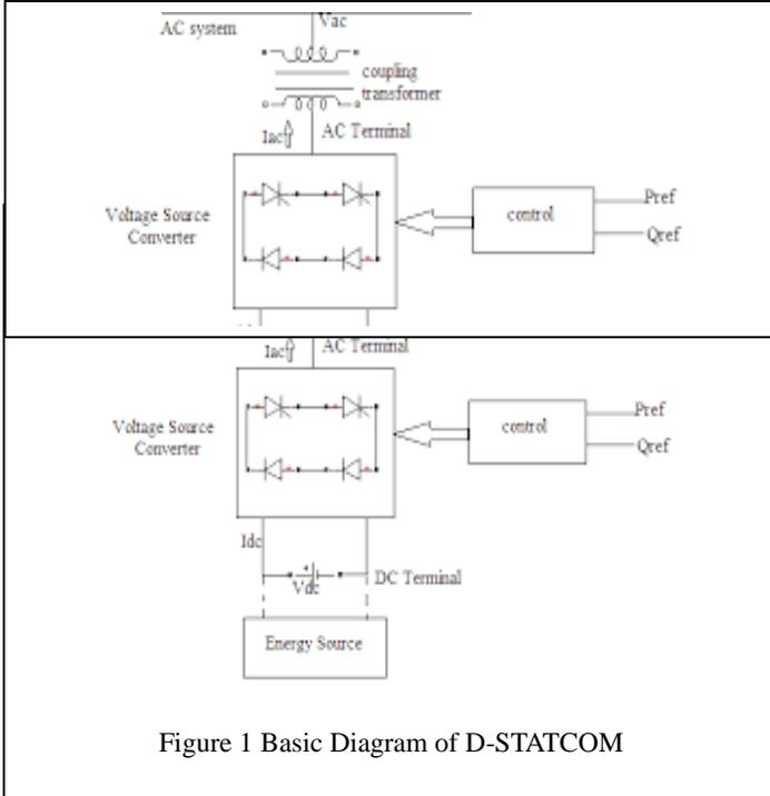
Figure 1 Basic Diagram of D-STATCOM
