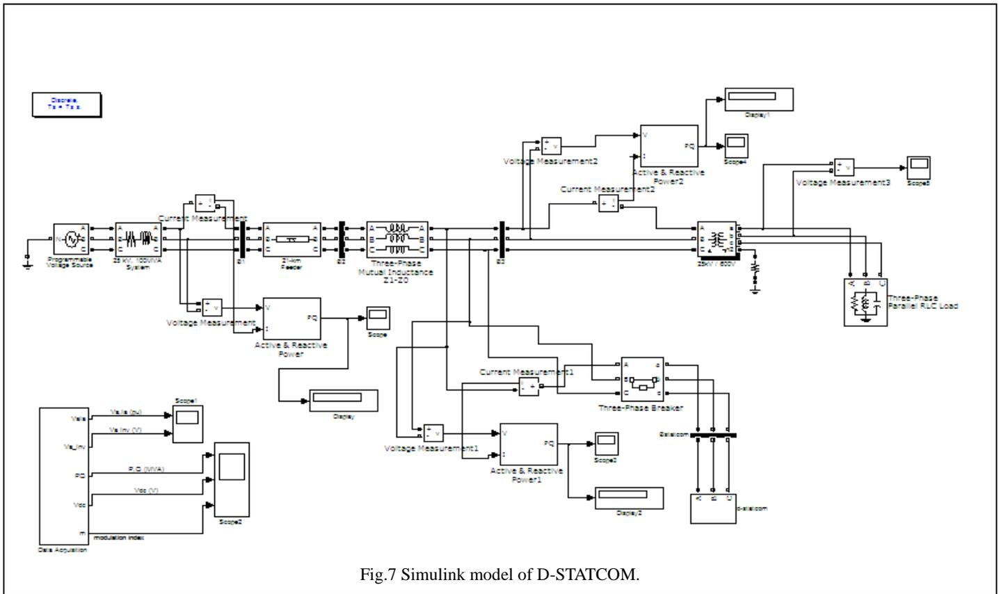
Fig.7 Simulink model of D-STATCOM.
