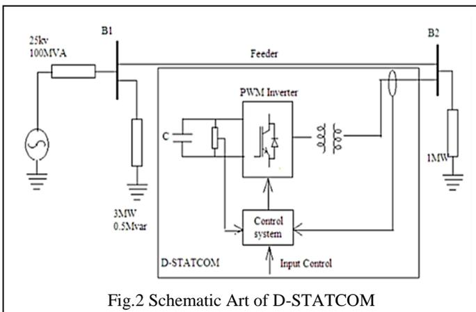
Fig.2 Schematic Art of D-STATCOM
