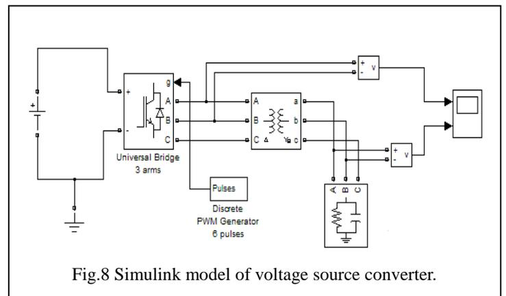
Fig.8 Simulink model of voltage source converter.
