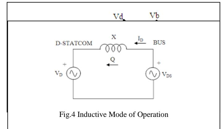
Fig.4 Inductive Mode of Operation
