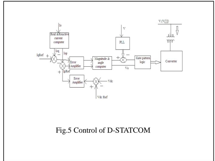
Fig.5 Control of D-STATCOM
