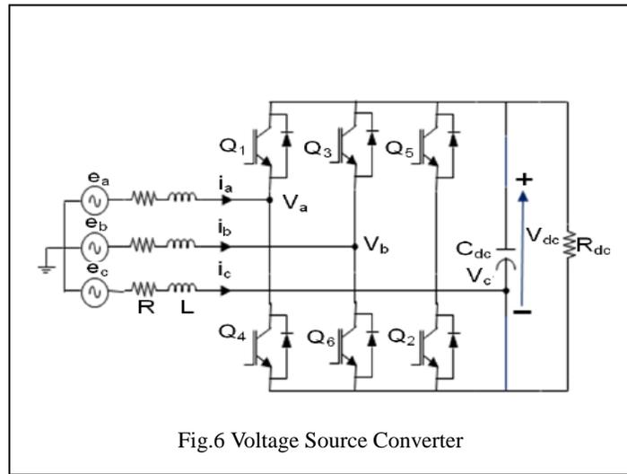
Fig.6 Voltage Source Converter
