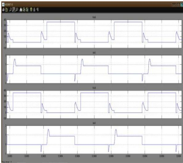
Fig.7 Voltage( $V_{ds6}$  &  $V_{ds8}$ ) and Current( $I_{ds6}$  &  $I_{ds8}$ ) waveform of MOSFET during Buck converter mode of operation.
