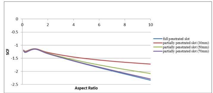
Fig. 7 Variations of SCF for full and partial penetrated the slot with different aspect ratio.
