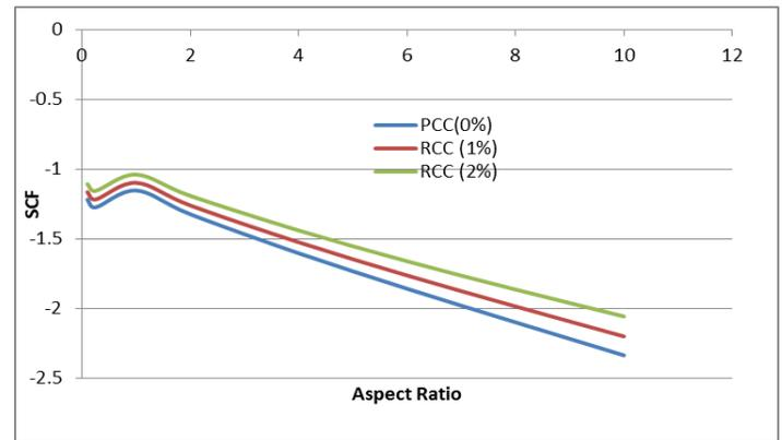
Fig. 8 Variations of SCF for full penetrated slot with different percentage of reinforcement.
