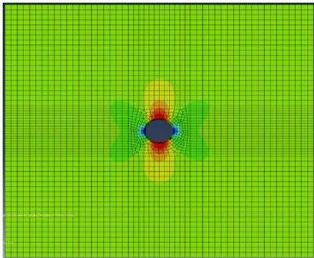
Fig. 2 Stress pattern on the slab with the hole
