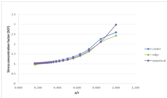
Fig. 3 Comparison of SCF with analytical study
