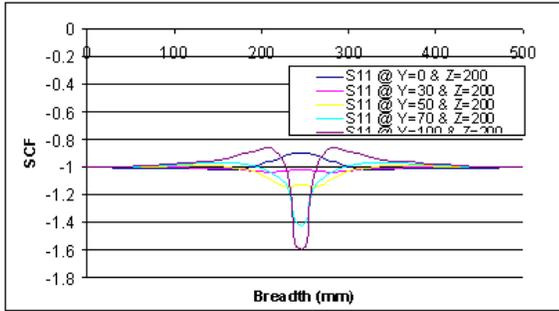
Fig. 10 Variations of stress at different locations (thickness) for Typ. Partially penetrated the slot (PCC).
