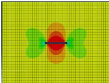
Fig. 4 Stress pattern on the slab with the rectangular the slot
