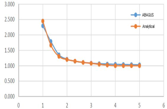
Fig. 5 Comparison of SCF with analytical study
