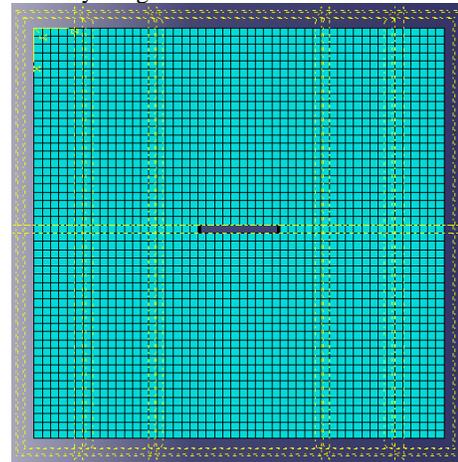
Fig. 6 FE model of the slab with the rectangular the slot
