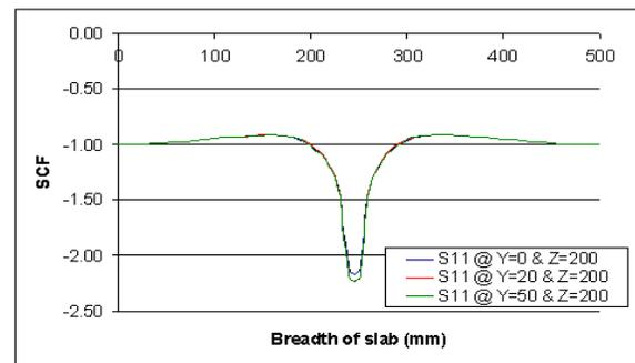
Fig. 9 Variations of stress at different locations (thickness) for full penetrated the slot (PCC).
