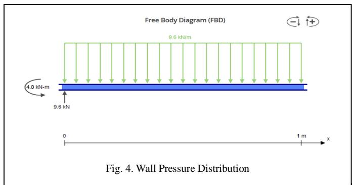
Fig. 4. Wall Pressure Distribution
