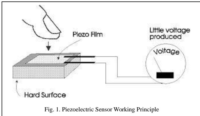
Fig. 1. Piezoelectric Sensor Working Principle
