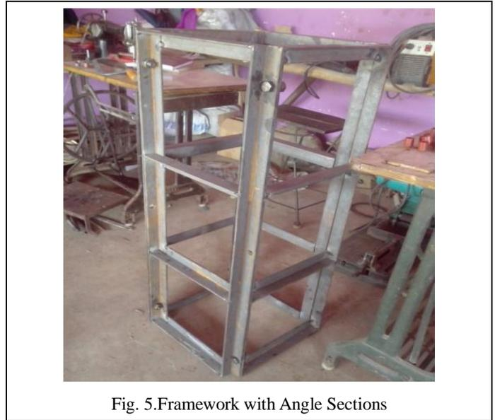
Fig. 5. Framework with Angle Sections
