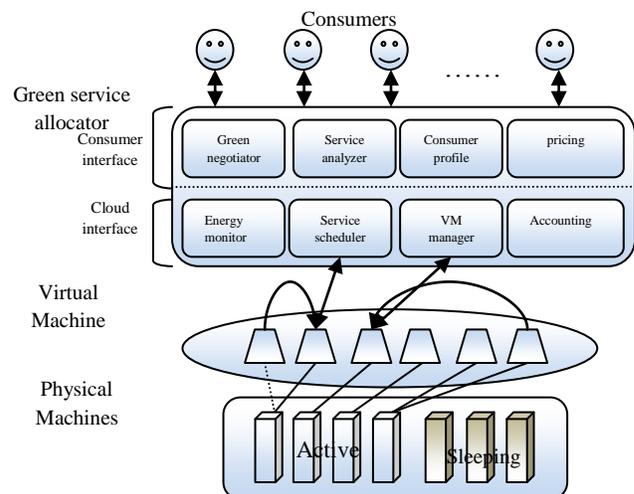
Fig.1: Architecture of a green cloud computing environment
