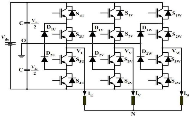
Figure 3 Three -level Neutral Point Clamped topology
