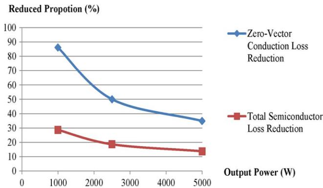
Figure 5 conduction and semiconductor loss reduction
