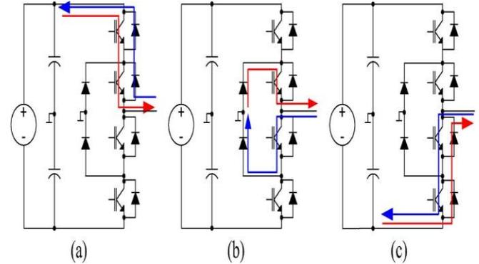
Figure 4 Current paths of conventional I-type 3L-NPC leg. (a) 1100. (b) 0110. (c) 0011.
