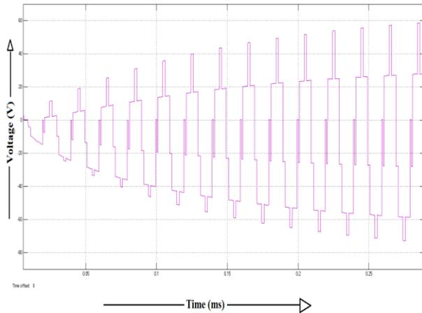
Figure 5 Inverter Side Output Voltage
