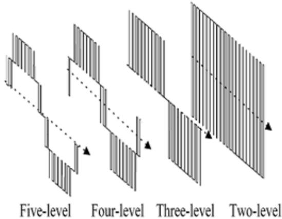
Figure 2 Waveforms of Multilevel inverter
