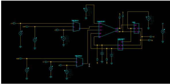
Fig. 4. Design of an offset cancelled comparator with time domain bulk-tuned offset cancellation. In this the MUX selects the input signals for different operation modes. The comparator compares the two input signal and generates the corresponding output signal. The phase detector senses the delay from the comparator outputs and drives a charge pump. The charge pump changes the body voltages of the input pair stored in Cb+ and Cb-, and cancels the offset.
