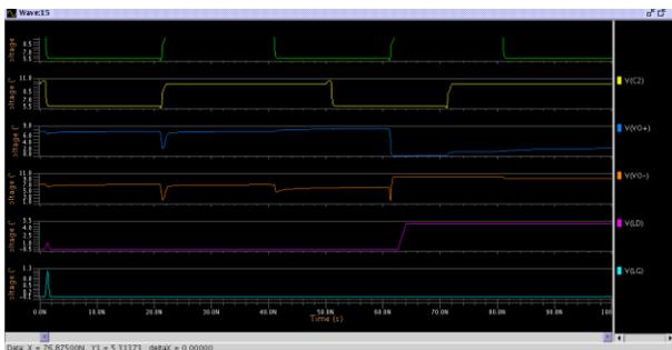
Fig. 5. Output waveform of the comparator with offset cancellation circuitry. In this due to the offset, the falling edge of V<sub>O+</sub> leads the V<sub>O-</sub>. So that the phase detector senses this delay and generates pulses on lead signal pin. Similarly the lag signal is generated when V<sub>O+</sub> lags V<sub>O-</sub>.
