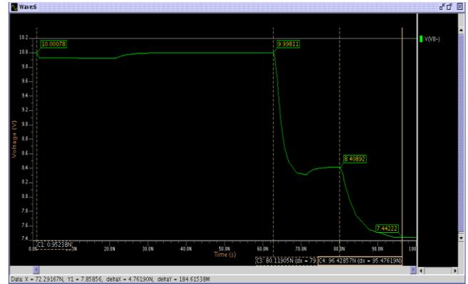
Fig. 6. The output waveform of the comparator body voltage calculation. If V<sub>O+</sub> leads V<sub>O-</sub>, then V<sub>b-</sub> will be decreased by while the other remains constant.
