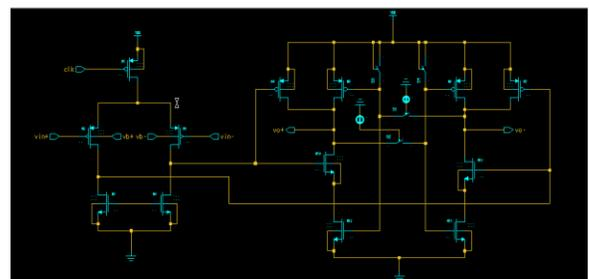
Fig. 3. Design of two stage comparator circuit with the offset cancellation circuitry. In this the switches s1 and s2 are open and the switches s3 and s4 are kept closed.
