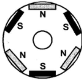
Figure1. Circular core with rectangular magnets embedded in the core.
