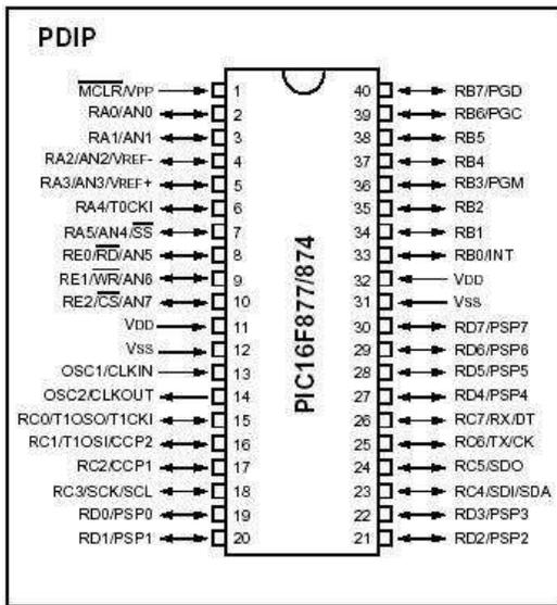
Fig 5 PIN CONFIGURATION OF PIC16F877
