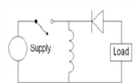
Fig 4 BUCK-BOOST CONVERTER
