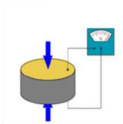
Fig 3 PIEZO ELECTRIC SENSOR
