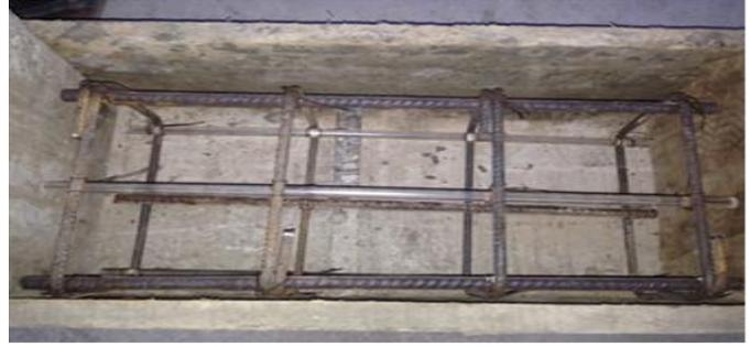
Fig.8 Reinforced with 50% Acrylic rods
