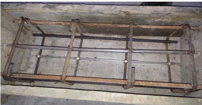
Fig.7 Reinforced with 25% Acrylic rods
