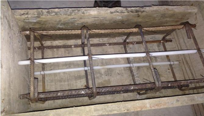
Fig.5 Reinforced with 25% polypropylene rods
