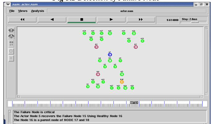
*Fig 5.3 Recovering a Failed Node*
