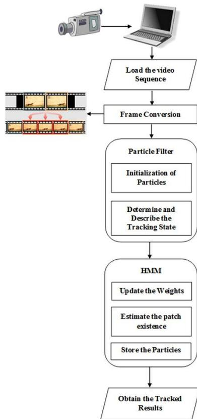
Figure 1. System Architecture of the Multi-Object Tracker
