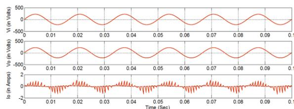
Fig.8. Simulation results of input and output line voltage and current for proposed method
