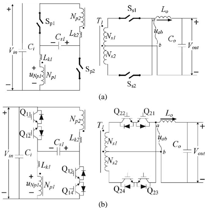
Fig.1 Proposed AHFL AC-AC converter (a) main circuit (b) realization of bi-directional switches
