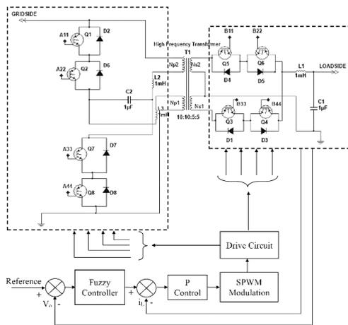
Fig.5 Typical system configuration with proposed IHFL AC-AC converter for voltage compensation
