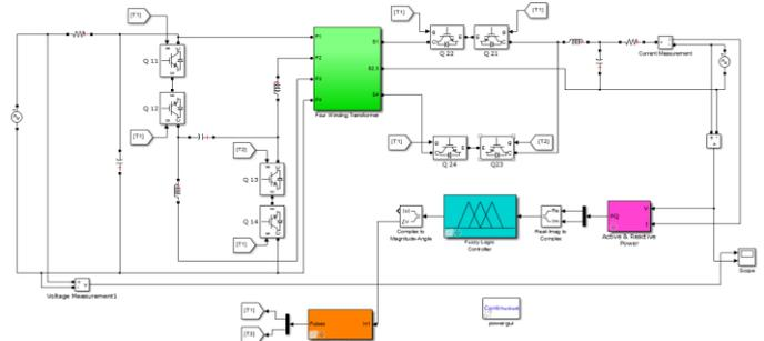
Fig. 6 Simulink Diagram of Proposed AHFL AC-AC Converter Scheme
