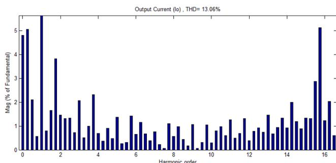
Fig.9. Simulation results of harmonic spectra of output line current for Proposed method
