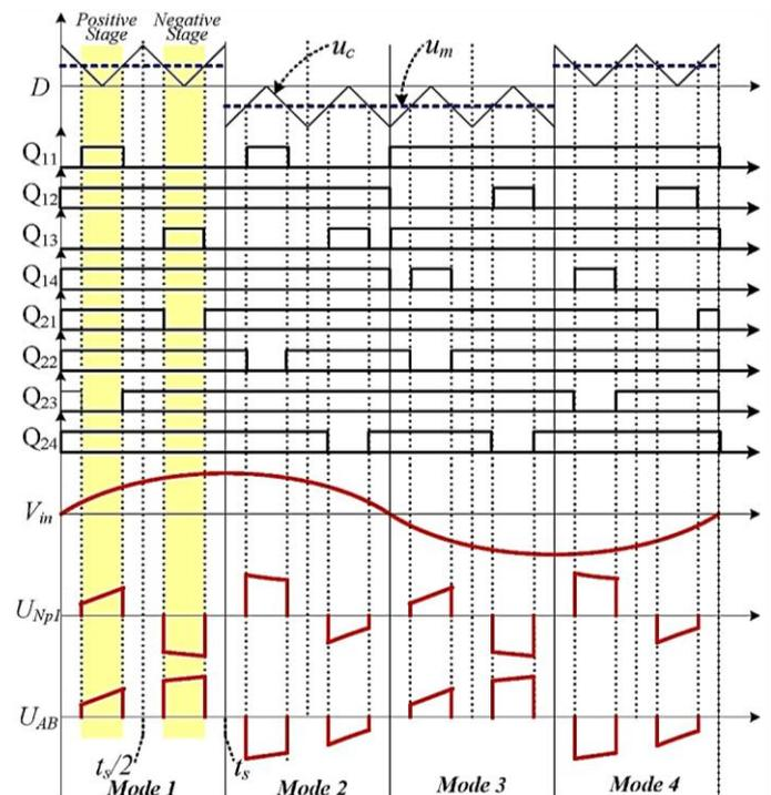
Fig.2 Demonstration of gate signals and crucial waveforms
