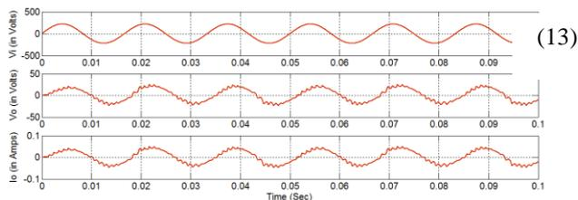
Fig.7. Simulation results of input and output line voltage and current for conventional method
