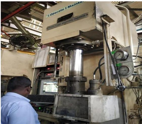
**FIG 1: pinion cage assembly bearing press with torque test**
