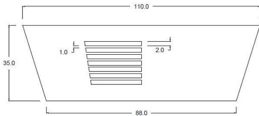
Figure 3: AutoCAD Drawing of Grooved Texturing
