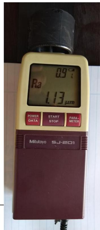
Figure 10: Surface roughness measurement for grooved texturing
