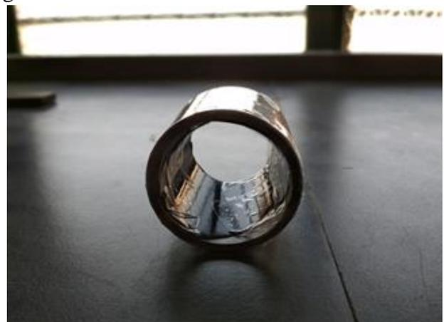
Figure 7: Bearing wrapped by radium-ready for etching
