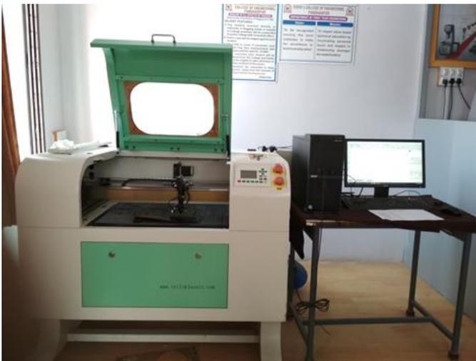
Figure 4: CO<sub>2</sub> Laser Cutting machine
