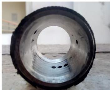
Figure 9: Bearing with grooved texturing
