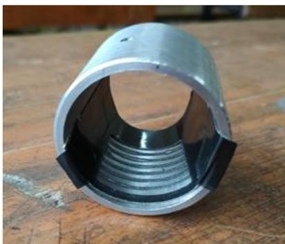
Figure 6: Radium maskant applied on the inner side of the bearing
