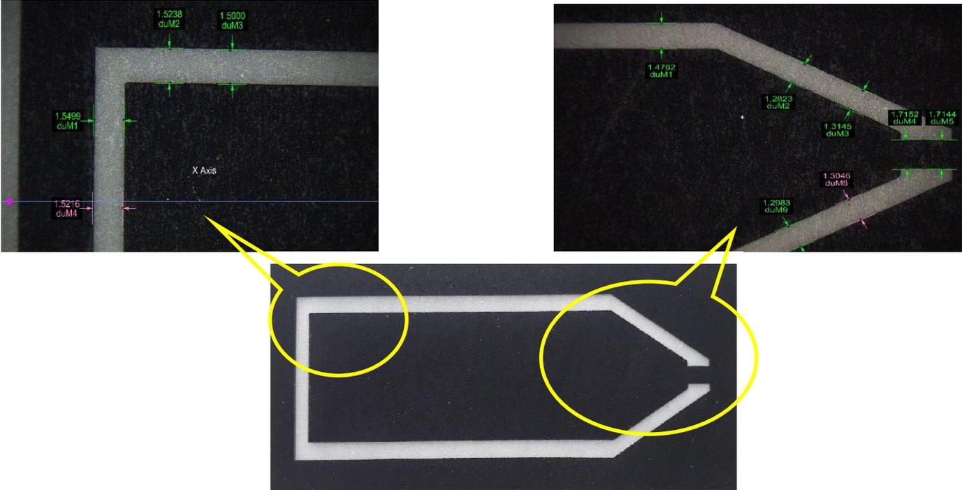
Figure 3: Characterization of the Photo tool
