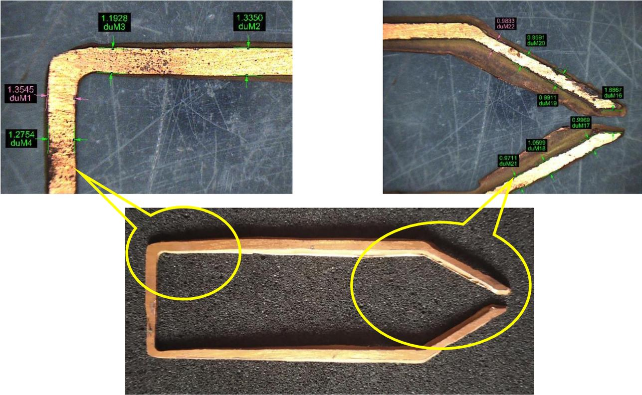
Figure 4: Characterization of fabricated Compliant Mechanism
