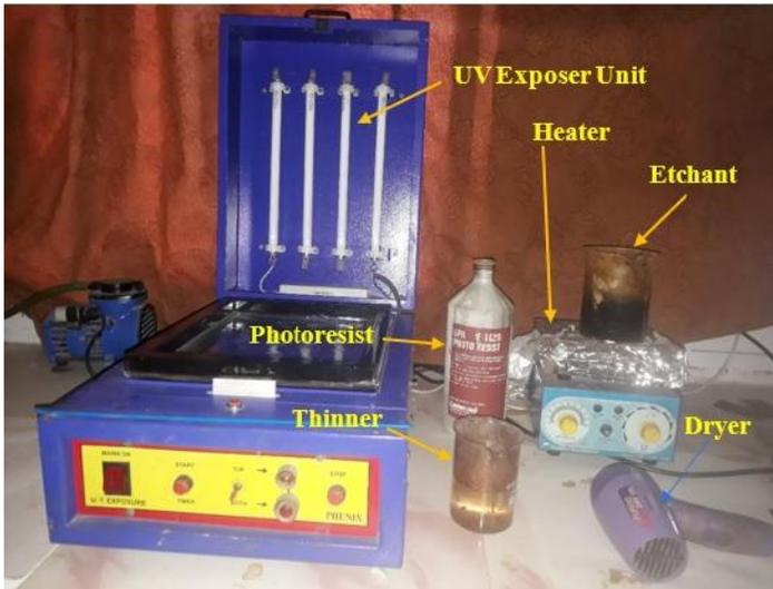
Figure 1: Photo chemical machining Setup
