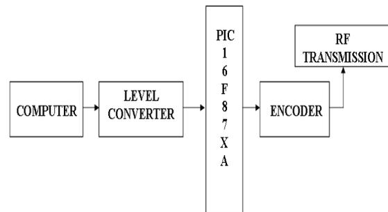
Fig 2.1 Block Diagram of EN UNIT
