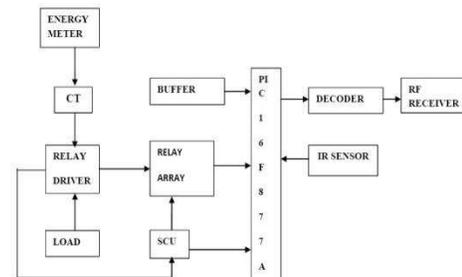
Fig.3.2: Block diagram of residential unit
