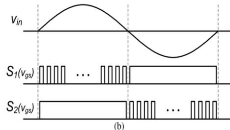
Fig .5 Gate signal for S<sub>1</sub> and S<sub>2</sub>
