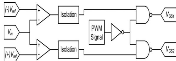
Fig. 4 Input voltage detecting circuit block diagram
