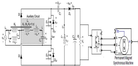
Fig.1. Proposed bridgeless SEPIC converter
