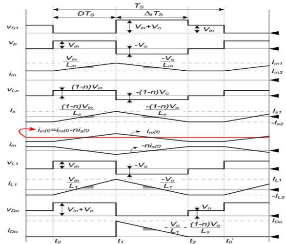
Fig . 3 Waveforms of the proposed converter
