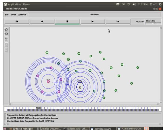
Fig 4 Figure represents Steady State phase of LEACH protocol
