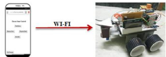
figure 7. Smart phone wi-fi controlled the robot
