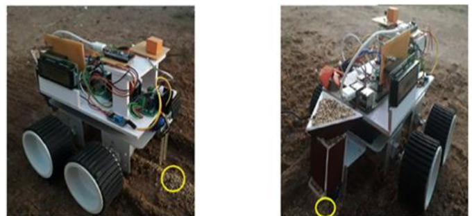
figure 4. experimentation and results for seed dispenser system
