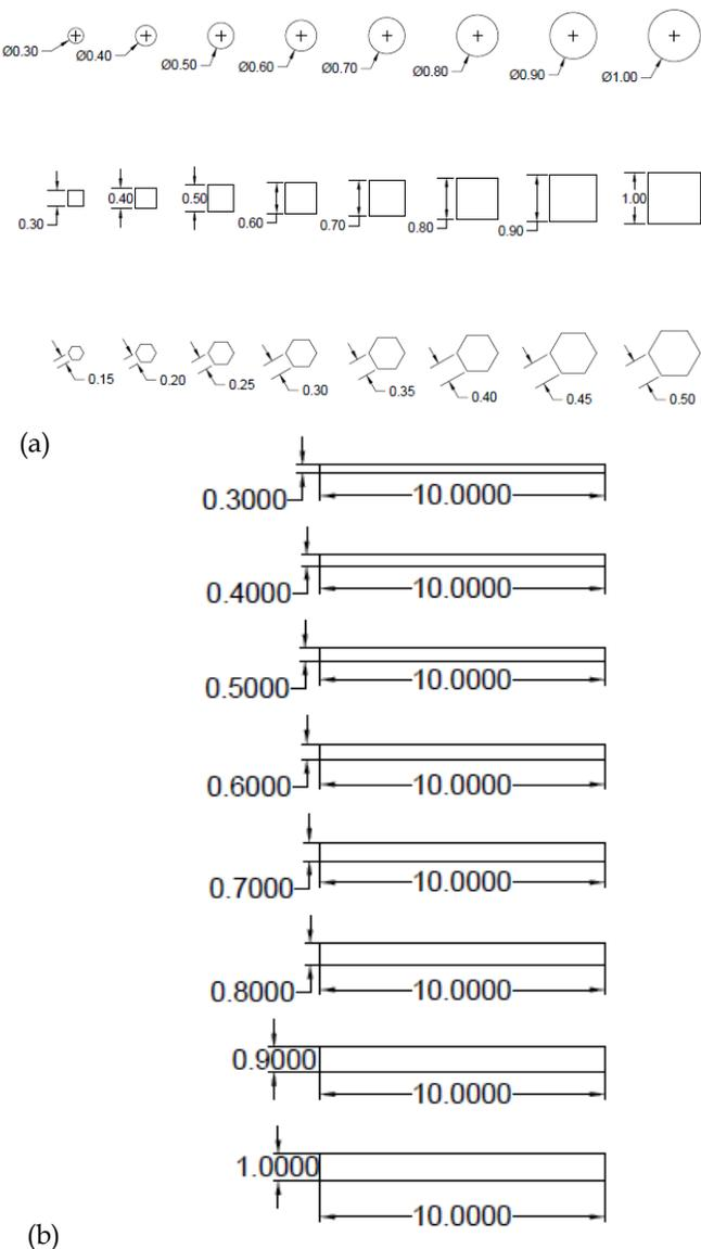
Figure 1: CAD Geometry for (a) Microfeatures (b) Straight channels
