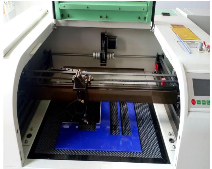
Figure 2: Laser Cutting Machine
