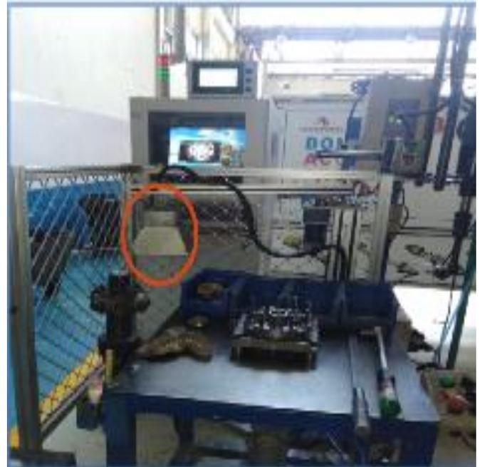
image found to be defect, displays the defect location and then it locks the next process.
