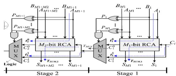
Fig. 1 structure of conventional carry skip adder (CSKA)
