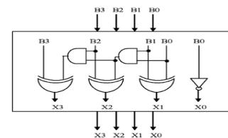
Fig.3 4-bit binary to excess converter
