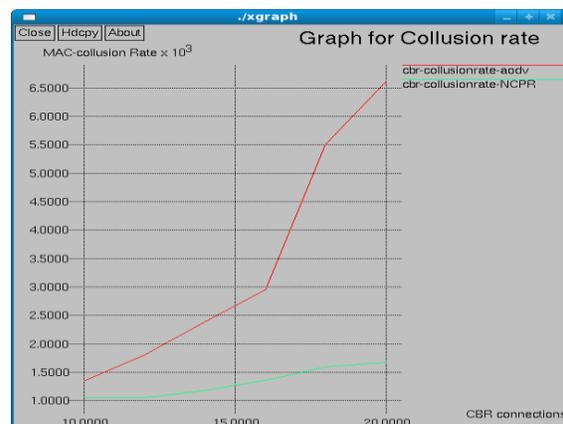
Figure 2: Performance Analysis for Collision Rate between AODV Vs. NCPR
