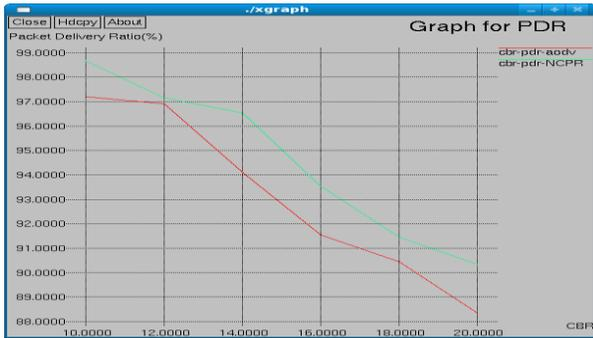
Figure 3: Performance Analysis for Packet Delivery Ratio between AODV Vs. NCPR
