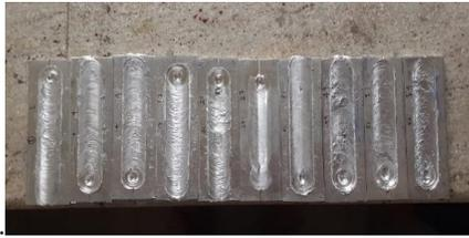
Fig. 7 Processed surfaces of the AA7075
