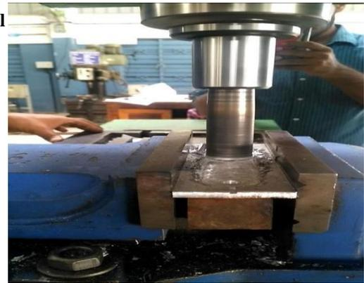
Fig. 4. Experimental setup of FSP
