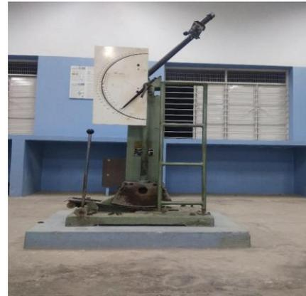
**Fig. 6 Impact strength tester**
