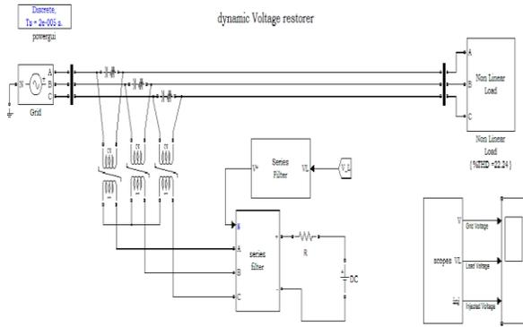
Fig 5 Simulation Diagram of dynamic voltage restorer
