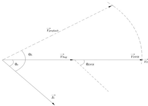
Fig 3 In-phase Compensation
