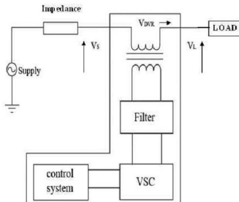
Fig 2 Block Diagram of DVR
