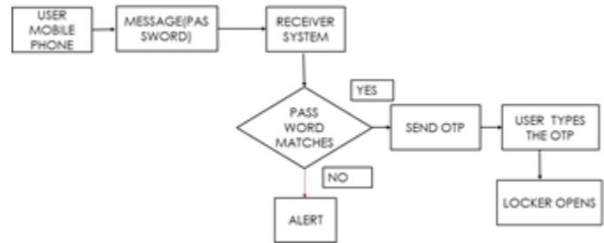
Fig 2.1 shows the block diagram of the basic block diagram of the working of this method
