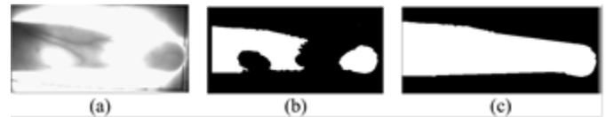
Fig 1.4 (a) Acquired finger vein image. (b) ROI mask from (a). (c) ROI mask after refinement. [1]
